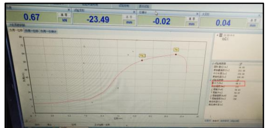
2. Pull-Out Test of Adit HSR M16x80
