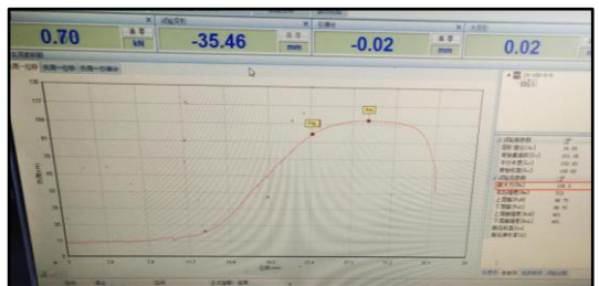
4. Pull-Out Test of Adit HSR M24x100
